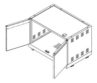
Cabinet connection: Connect each cabinet together by installing the screws if needed.
